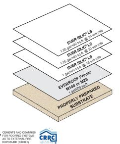
The EVER-SILIC<sup>®</sup> SYSTEM provides tenacious adhesion with an existing roof system to form a monolithic membrane. The result is a CRRC rated system that exceeds all Title 24 requirements.
